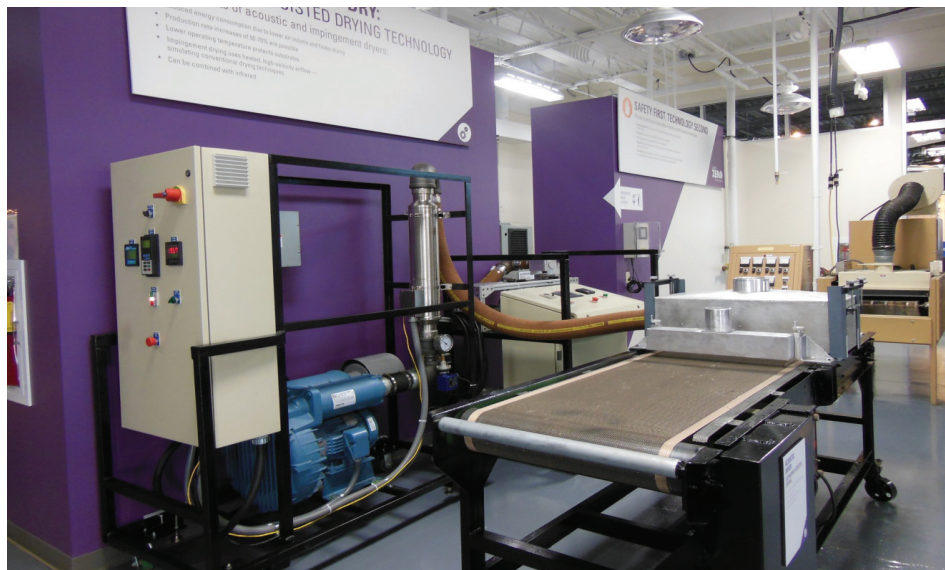
FIGURE 3. Acoustic three-slot commercial dryer used for pilot trials
